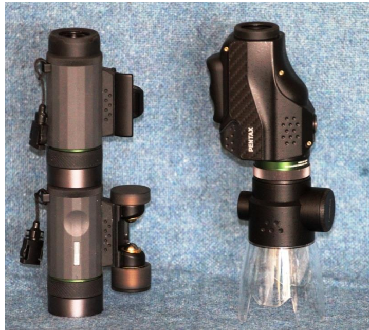
Fig 12. Left: Two halves of the Asahi Pentax 4x20 binocular coupled to form a 17x20 monocular telescope. Right: The Asahi Pentax 6x21 roof prism monocular converted into a microscope with built-in illumination (LED lights).
