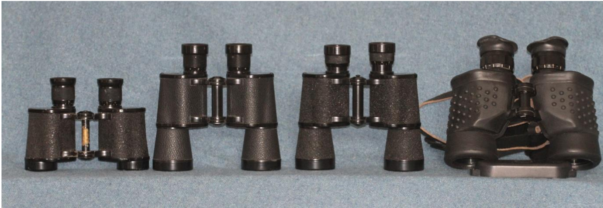
Left to right: PZO 6x30, PZO 8x40, PZO 11x40 and PZO 7x45C, all with Porro prisms.
