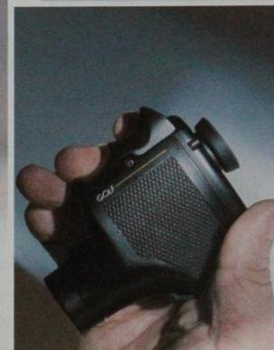
**Bynolyt 5x20 monocular with 3x enlarging magnifier.
