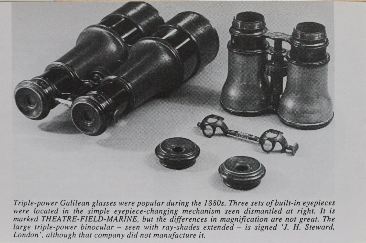
*Triple-power Galilean glasses were popular during the 1880s. Three sets of built-in eyepieces were located in the simple eyepiece-changing mechanism seen dismantled at right. It is marked THEATRE-FIELD-MARINE, but the differences in magnification are not great. The large triple-power binocular – seen with ray-shades extended – is signed 'J. H. Steward, London', although that company did not manufacture it.*
