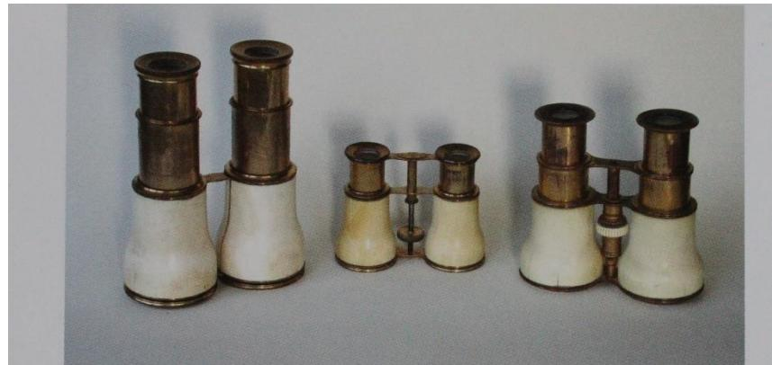
**Fig. 2** Three very early ivory binoculars from the period from 1825–1830. The left specimen is one of the first serially produced two-eye binoculars (Voigtländer, patent in 1823). The centre binoculars dated 1825 (also from Voigtländer) is perhaps the oldest known extant instrument with a centre-mounted focusing mechanism. Right: Petitpierre, Berlin, around 1830/40. Centre-mounted focusing mechanism and screw focus for the ocular supports.
